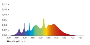
The test protocol reveals that the fluorescent lamp JUST daylight 5000 proGraphic fulfills the strict criteria for standardized lighting according to ISO 3664:2009.
